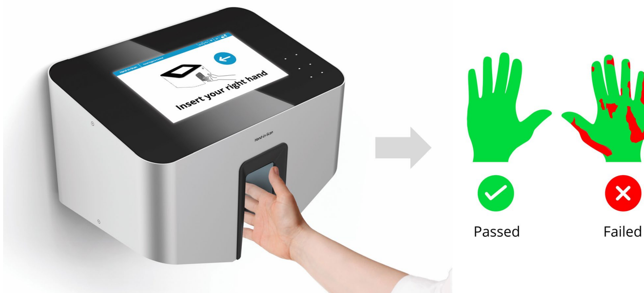
Fig. 2 Measurements using the Semmelweis System, where green indicates handrub-covered areas, red indicates non-covered areas determined by an AI algorithm, based on image analysis performed on recorded hands, treated with an UV-dyed alcohol-based solution. (Image credit: HandInScan Zrt)
