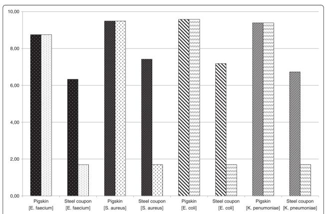
**Figure 1 Pre- and post-exposure populations of challenge microorganisms following transfer procedures.** Left bars: uncoated glove, right bars: coated glove.
