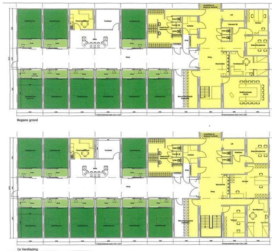
Fig. 2 Plan of the new ICU consisting of two identical floors with 9 patient rooms each. Single patient rooms with anteroom are indicated by dark green and light green, respectively
